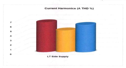
As detailed above, the voltage harmonics levels were around 2.92 - 3.25 % and the levels of the current harmonics were 4.74 - 6.53%. The Overall Voltage harmonics and the current harmonics are within limits.
